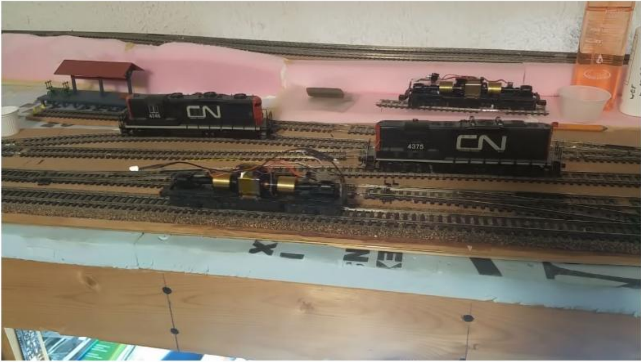
DCC decoder install in an Athearn locomotive
